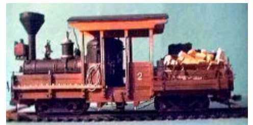
Another of Cache Creek Scale Models highly detailed On30 show models. This loco has a wood frame and the motor inside the tank has a drive line to a transmission with drive lines to both the front and rear trucks. MDC trucks & gear box. Emmett J Brannan Photo.
