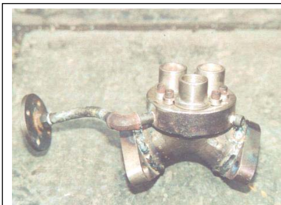
Above and Right: The assembled blast pipe components. The blower is incorporated into the main flange with 3 jets located just outside the retaining screws. Blast nozzles are quickly removed for adjustment or cleaning the assembly.
