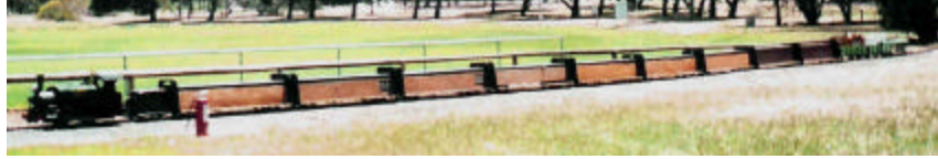
Photo 9: show the modified locomotive (with obligatory summertime fire extinguisher close by) with the standard test load behind. Weighing in at approximately 1.25t, a modest but adequate load for this loco.
